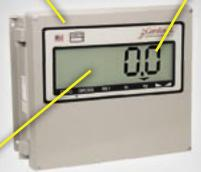
Display.....transflective LCD with light sensitive backlighting Display Capacity.....-99999 to 999999 Backlight Type.....Photo detector controlled CCFL, 10,000 Hr Life Annunciators...... 6 (Zero, Gross, Net, lb, kg and Motion) Ambient Light Levels ..... total darkness to direct sun **Power Input.....** 3 wire, 95 to 264 VAC, 60 Hz (10' / 3 m cable furnished) Enclosure Rating.....NEMA 4/IP65
